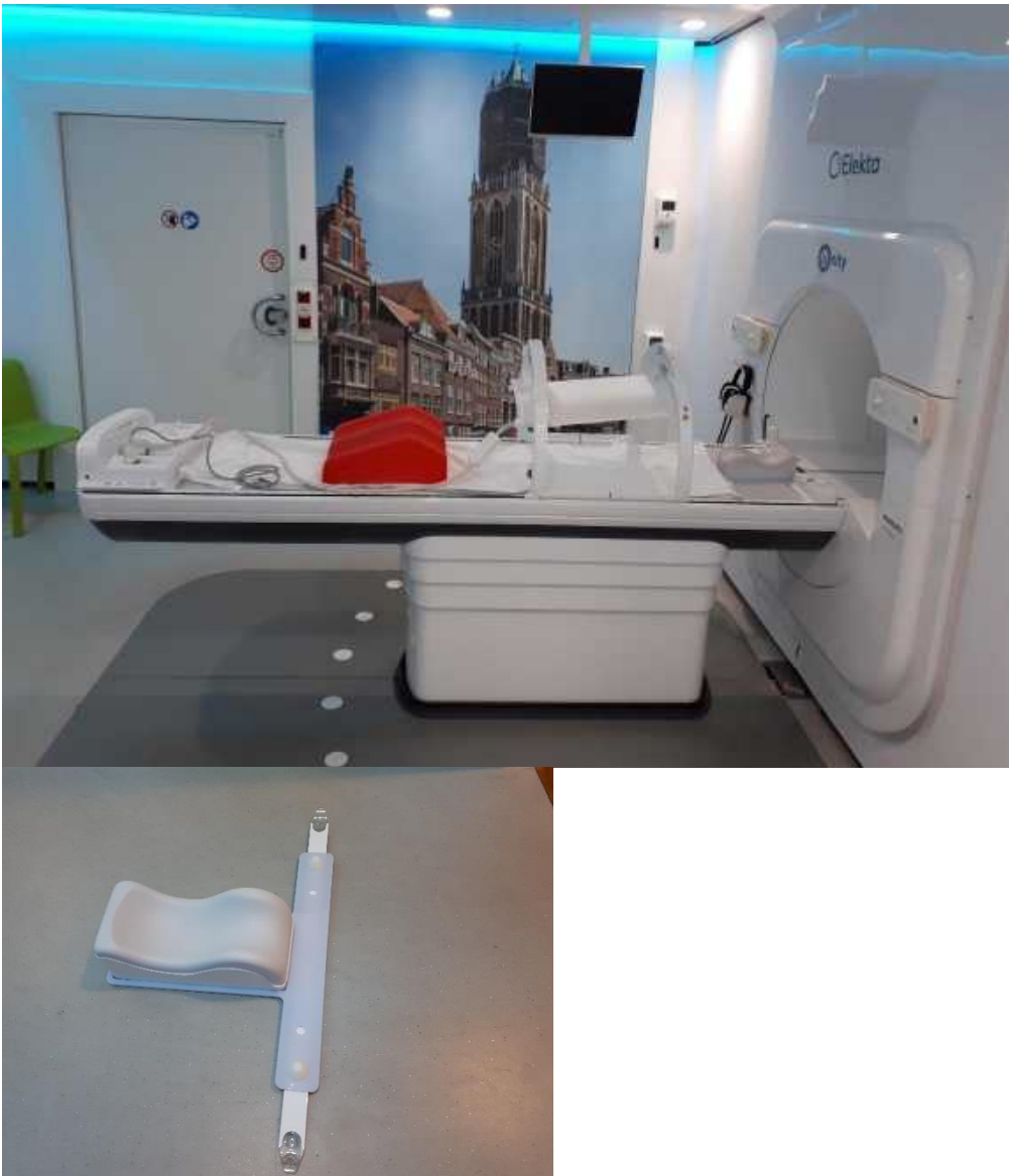
Courtesy of UMC Utrecht – Unity Elekta MR-Linac. Used devices: Headrest M with Headrest indexing adapter attached to indexing bar, KneeSupport™ foam, anterior Elekta coil bridge, headphones and earplugs, emergency squeeze bulb, optional: prism glasses and BOLD TV screen
